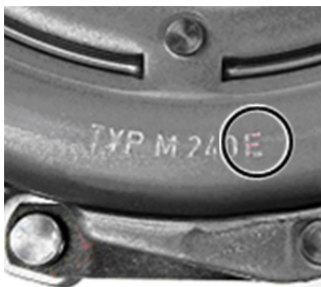
Fig. 2: All Xtend clutches are marked with the suffix code symbol E , for example: M 240 E
