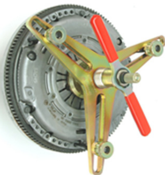
Fig. 3: Clamping device with centering pin
