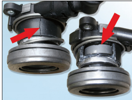
Image 5: CSC damaged by improper installation
